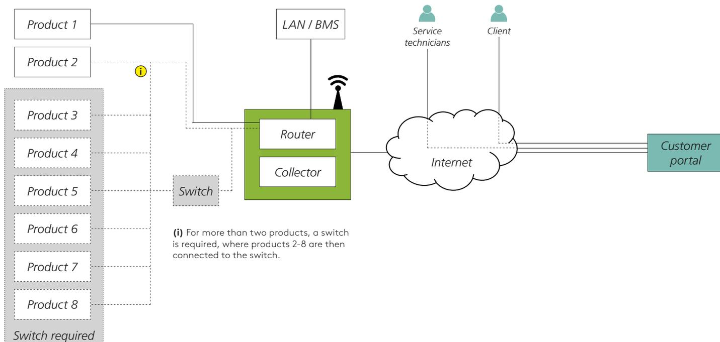
Fig. 6: System overview and connections.
