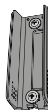
Figure 4. Back-piece Screw mounting on the wall, screw max. Ø4.5 mm, min. length 20 mm, screws not supplied.
