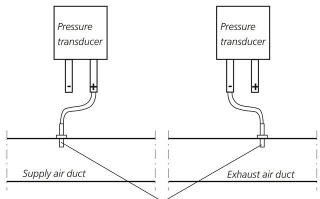
N.B! In some cases you might need to cut the measurement tapplings to shorten them. They should not protrude more than 10 mm from the inner wall inside the duct.
